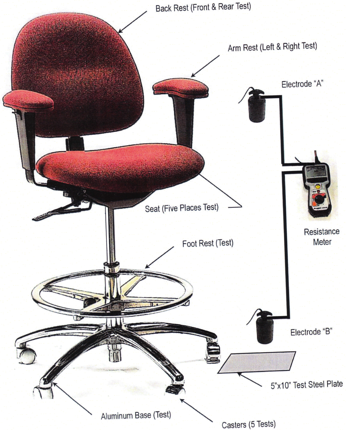
FIGURE 1: RESISTANCE TO GROUNDABLE POINT TEST POSITIONS
